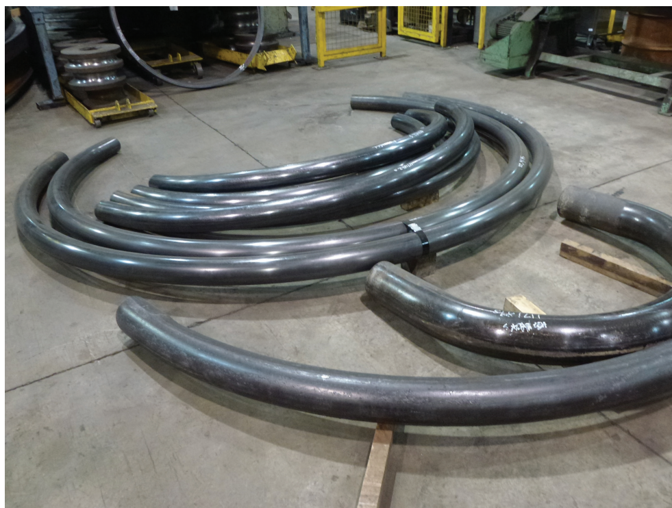
Fig. 1-15. Stocky, round HSS, tightly curved by three-roll cold bending.
