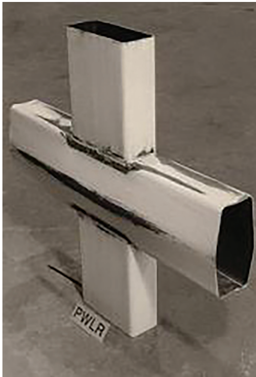
(a) Cross-connection with web buckling
