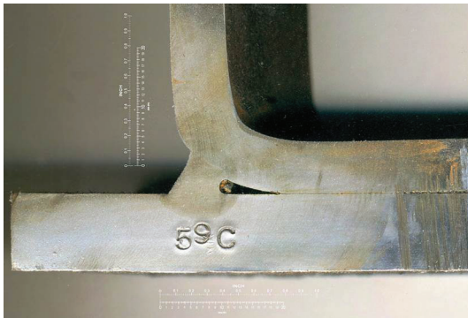
(a) Flare-bevel weld, cross section
