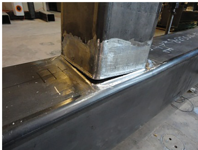
Fig. 3-16. Typical fillet weld fracture for an HSS-to-HSS 90^\circ T-connection under branch in-plane bending.
