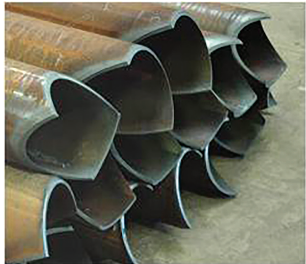
(b) Tube ends prepared with saddle cuts for fabrication
