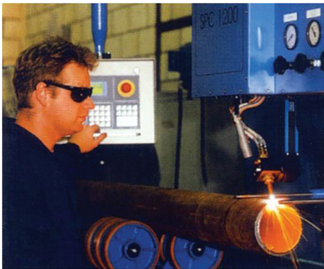
(a) Cutting and beveling while rotating the tube
