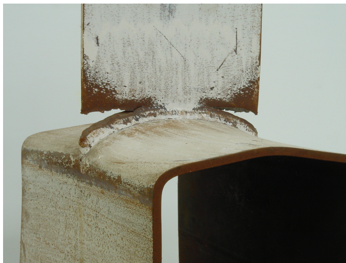
(a) Tension-loaded transverse branch plate at failure
