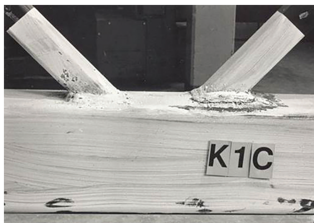
(b) K-connection with concrete-filled chord
