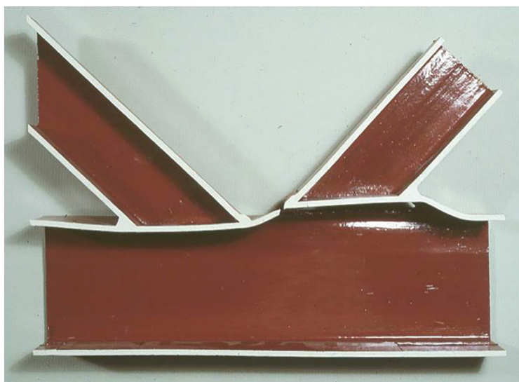
Fig. 2-6. Longitudinal cross section through an HSS K-connection at ultimate load.
