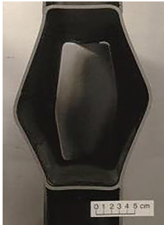
(b) Cross section through connection shown in part (a)
