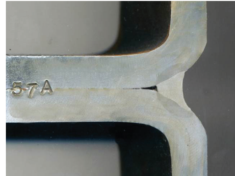
(b) Flare-V weld, cross section
