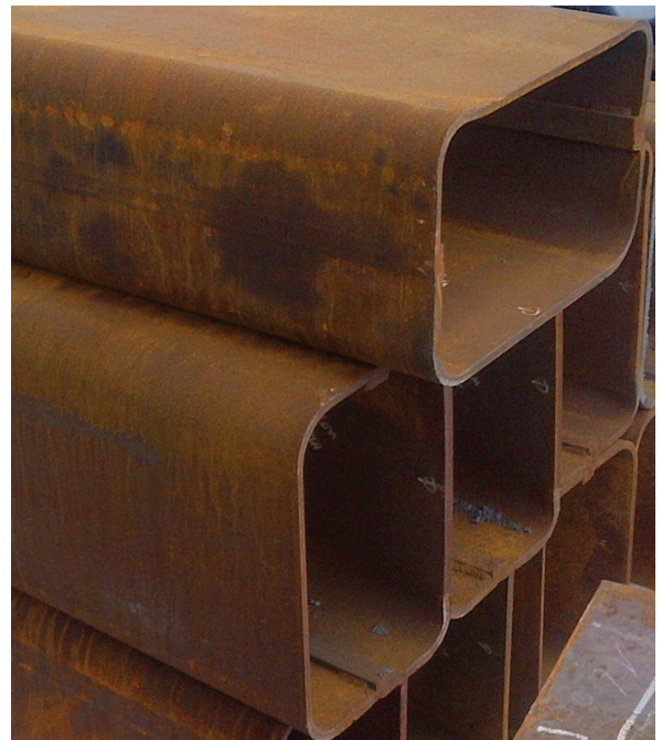
Fig. 1-12. ASTM A1065/A1065M Type 1 HSS (SAW C-shapes, with backing bars to the short sides, left in place) (photos courtesy of Valmont Industries).
