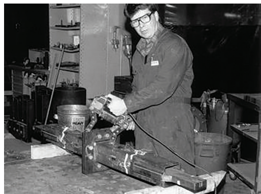
Fig. 3-11. Magnetic-particle testing of an HSS connection.
