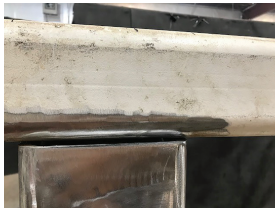
Fig. 3-7. Matched-width T-connection with large fit-up gap.
