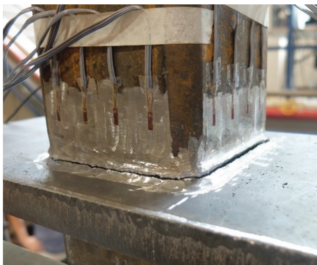
Fig. 3-1. Fillet weld fracture tests on square and round HSS-to-rigid end-plate connections.
