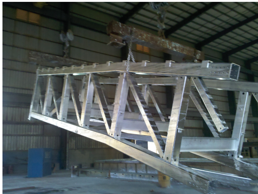
Fig. 1-17. HSS truss with drain/vent holes after hot-dip galvanizing (photo courtesy of American Galvanizers Association).
