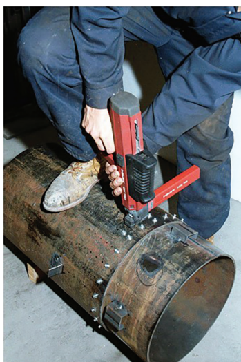
Fig. 4-9. Fastening two mating HSS together.
