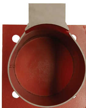
(a) Post-test bisection of a transverse plate connection experiment
