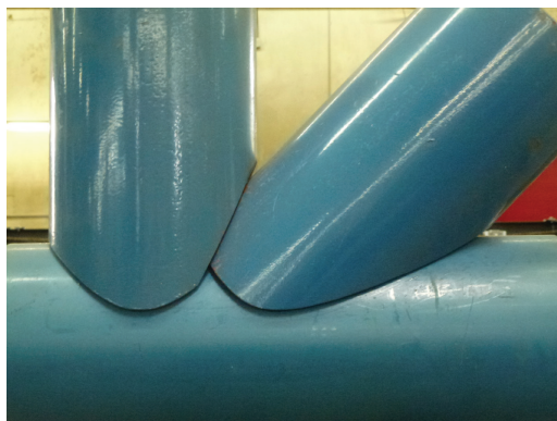
(a) Partially overlapped round HSS K-connection
