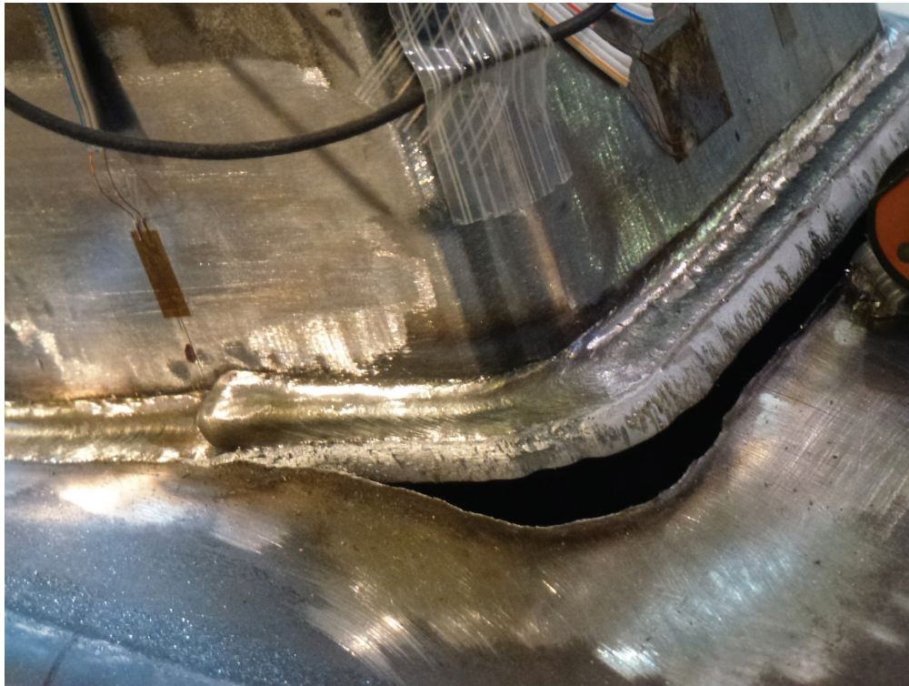
Fig. 10-5. Laboratory test of a rectangular HSS-to-HSS T-connection under branch in-plane bending (McFadden and Packer, 2014): failure by chord wall plastification followed by chord punching shear at ultimate moment ( \beta = 0.5 ).
