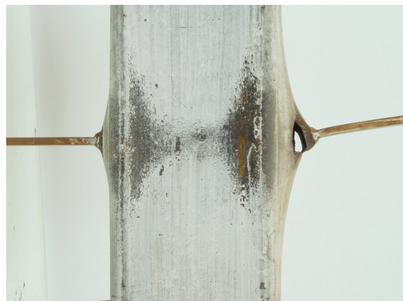
(b) Chord face plastification, combined with chord punching shear and local yielding of the chord side walls, for a transverse plate connection
