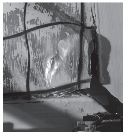
Fig. 2–16. Fracture of infill panel corner at 3.07 percent drift (Berman and Bruneau, 2003b).
