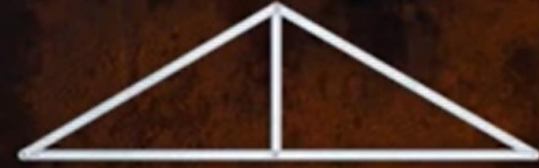
King Post roof truss
