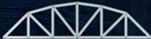
Parker bridge truss
