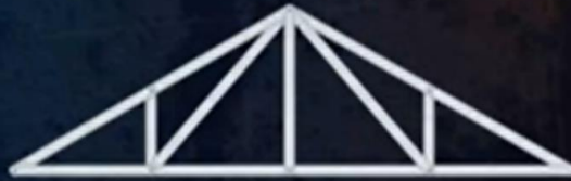
Pratt roof truss
