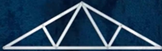
Fink roof truss
