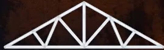
Modified Queen roof truss
