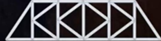
K bridge truss
