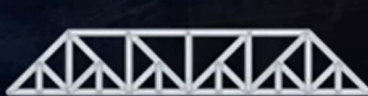
Baltimore bridge truss
