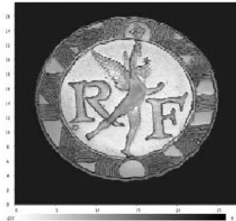
Figure 89 : C scan, 50 MHz, focalised beam
