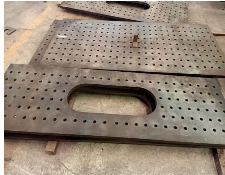
Fabrication : Drill Splice plate
